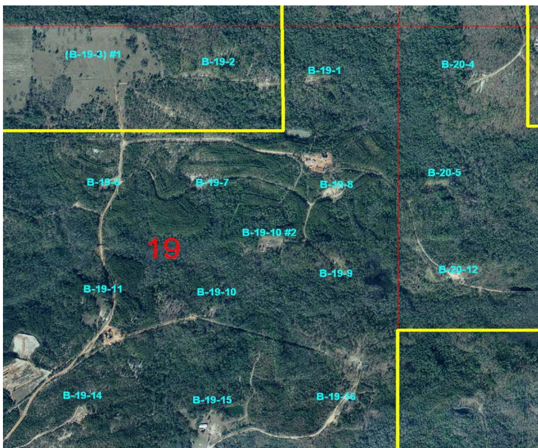
Figure 2.6.1. Aerial photograph of the Citronelle oil field in the vicinity of the test well pattern. The top edge of the photograph faces North. The test pattern consists of injector B-19-10 #2 and producers B-19-7, B-19-8, B-19-9, and B-19-11. Tank Battery B-19-8 is visible just to the Northwest of Well B-19-8. Tank Battery B-19-11 is to the South of Well B-19-11, between the roads.
